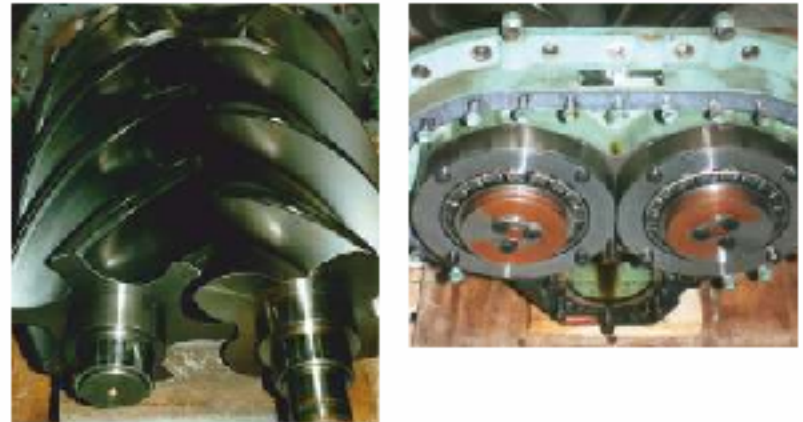
Sullair air compressor after 10.000 hrs. using Klüber Summit SH ® -46 without an oil change
