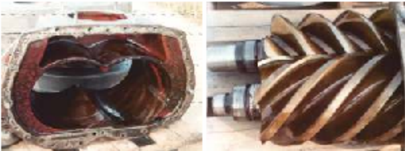
Petroleum lubricant used beyond the recommended oil drain interval (ODI)
