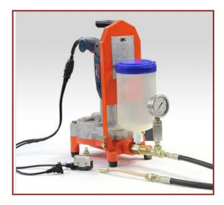
High pressure injection pump is ideally suited for grouting of epoxy/polyurethane grout materials. It's compact design enables easy handling on job sites and ensures efficient cracks filling in concrete.
