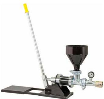
Portable hand operated grout pump comes on a skid with a 11 liter material holding hopper connected directly to the suction of the pump for a continuous pumping operation of water based cementitious grout.
